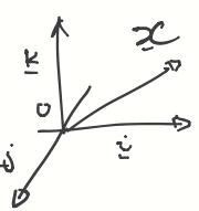
$$\underline{x} = (x_1, x_2, x_3) = x_1 \cdot \underline{i} + x_2 \cdot \underline{j} + x_3 \cdot \underline{k}$$
