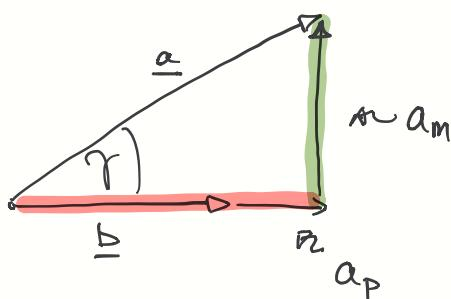
$$\bullet \underline{a}_p = \underbrace{\underline{a} \cdot \frac{\underline{b}}{|\underline{b}|}}_{|\underline{a}| \cdot \cos \gamma} * \frac{\underline{b}}{|\underline{b}|} = \frac{\underline{a} \cdot \underline{b}}{|\underline{b}|^2} * \underline{b} = \frac{1}{2} \underline{b} = (2, -1, 1)$$
