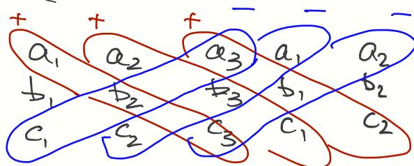
$$(\underline{a} \times \underline{b}) \cdot \underline{c} = a_1 b_2 c_3 + a_2 b_3 c_1 + a_3 b_1 c_2$$
